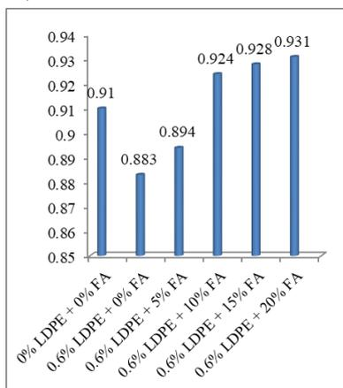
Fig. 1: Variation of compaction factor with fly ash content. Compaction factor test was used for determining the workability of fresh concrete. Bar chart has been plotted for
