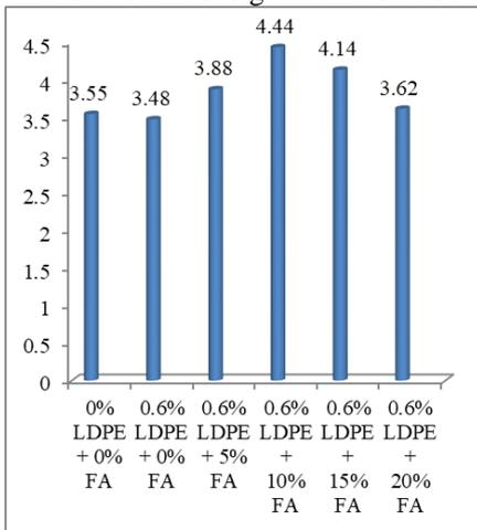
Fig. 3: Variation of Flexural strength with fly ash content
