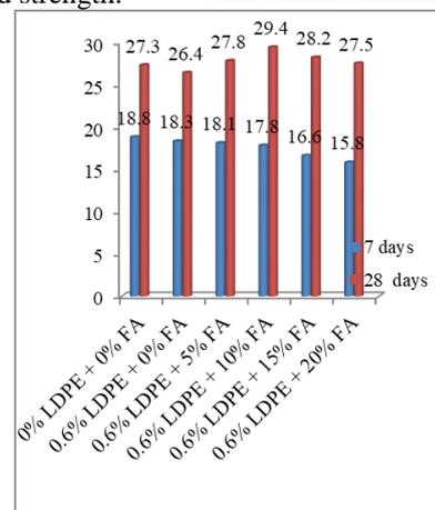
Fig. 2: Variation of Compressive strength with fly ash content
