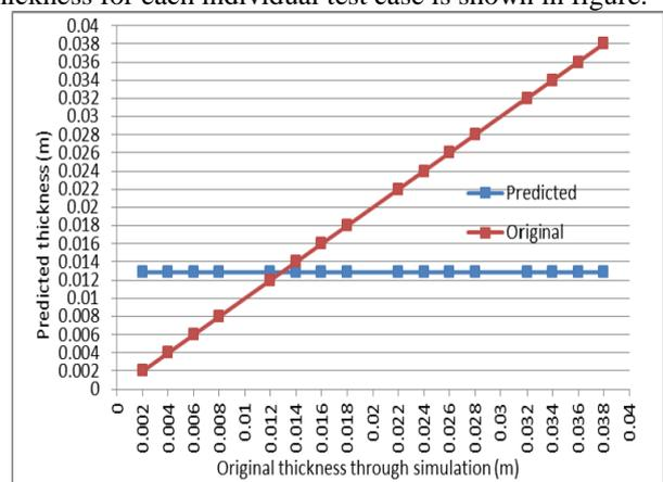
Fig. 4: Comparison between the original thickness during simulation and predicted thickness.
