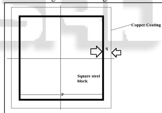
Fig. 1: The schematic representation of square steel block with copper coating.
