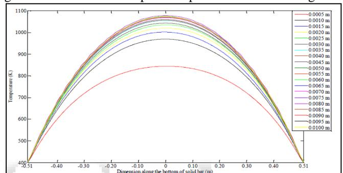
Fig. 3: For inner face, the start grid size with varying temperature profile.
