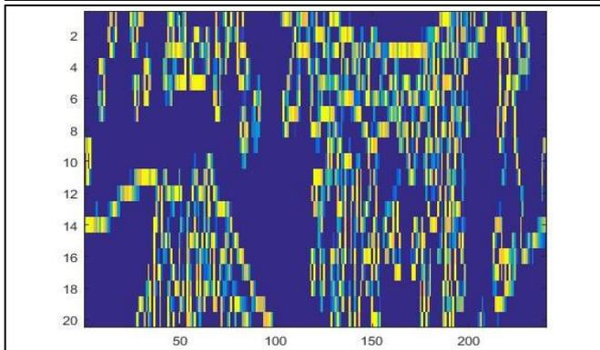
Fig. 6: Iris unwrapping into constant rectangular dimensions (Normalised template)
