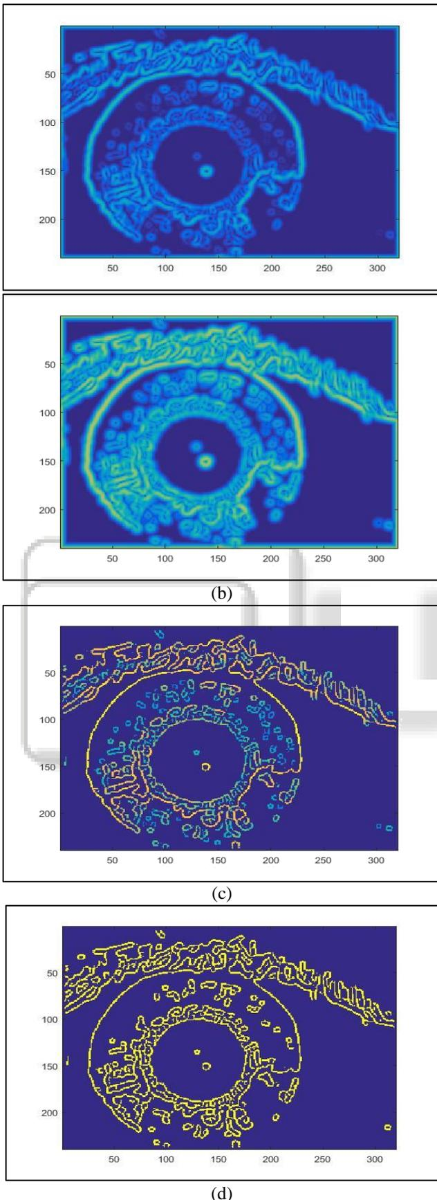
Fig. 2: The Edge Detection process: Images, in sequence, after (a) Canny Edge Detection, (b) Gamma Thresholding, (c) Non-Maximum Suppression and (d) Hysteresis Thresholding
