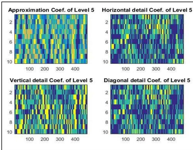
Fig. 8: DWT (Haar) Level 5 decomposition of the normalized image
