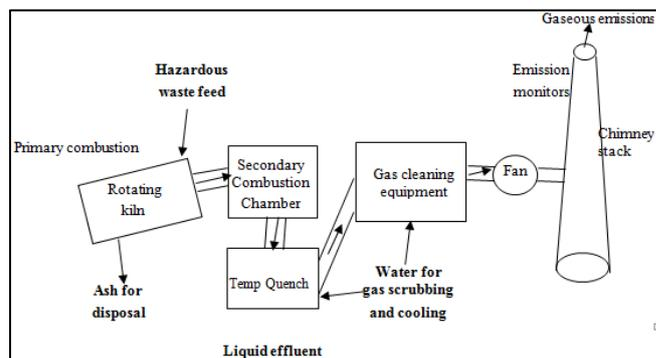
Fig. 2: High Temperature Incineration method
