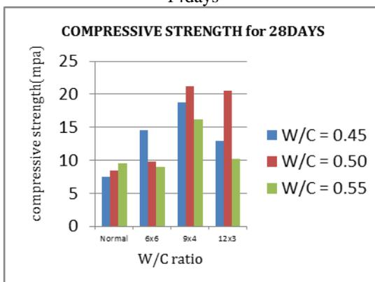
Fig. 5: shows compressive strength for 2% of fibers for 28days
