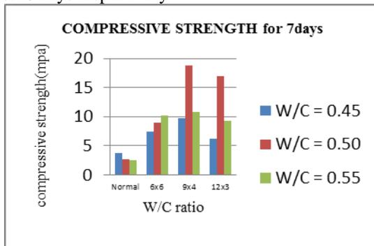
Fig. 3: shows compressive strength for 2% of fibers for 7days
