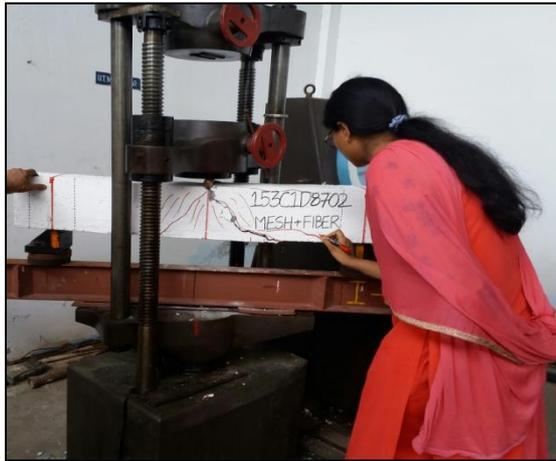
Fig. 15: shows crack pattern
