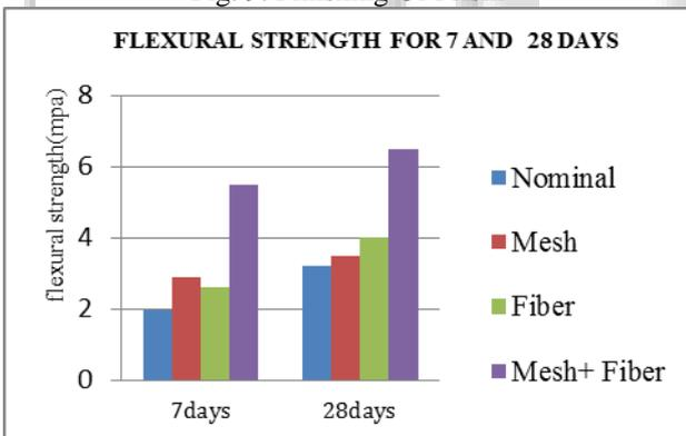
Fig. 10: shows flexural strength for optimum 4% of fibers for 7&28days
