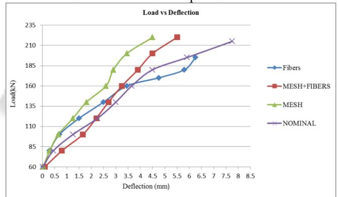
Fig. 13: shows Load VS deflection curve for 28 days
