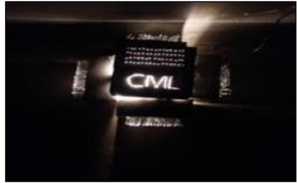
Fig. 12: Light transmitting block when placed in dark room
