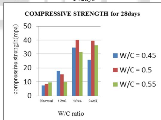
Fig. 8: shows compressive strength for 4% of fibers for 28days
