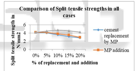
Fig. 12: Indicates the comparative result of split tensile strength in all three cases.
