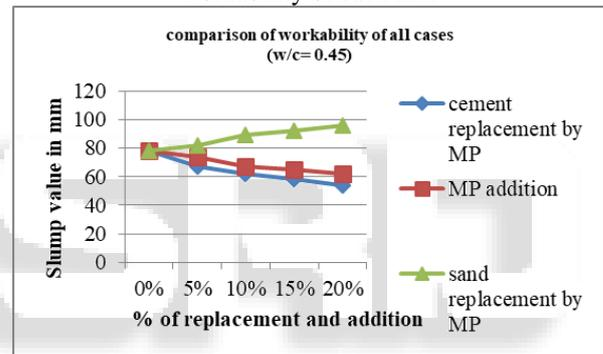
Fig. 3: Indicating the comparison of workability of concrete prepared for all of the three cases.
