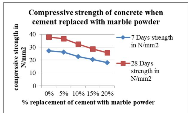
Fig. 4: Indicates the compressive strength of concrete when cement replaced with MP
