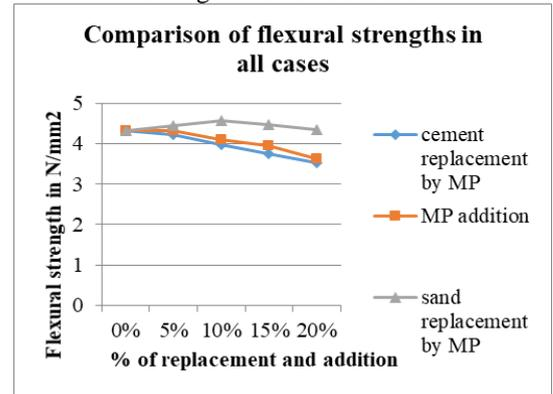
Fig. 11: Indicates the comparative result of flexural strength in all three cases.
