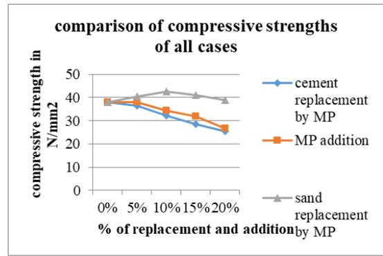
Fig. 10: Indicates the comparative result of compressive strength in all three cases.
