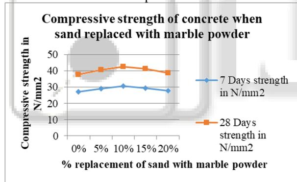
Fig. 8: Indicates the Compressive strength of concrete when sand replaced with marble powder.
