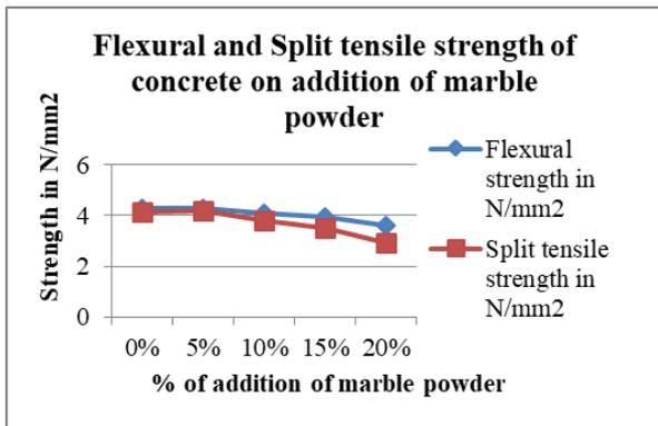
Fig. 7: Indicates the Flexural and split tensile strength of concrete on addition of MP to the standard mix.
