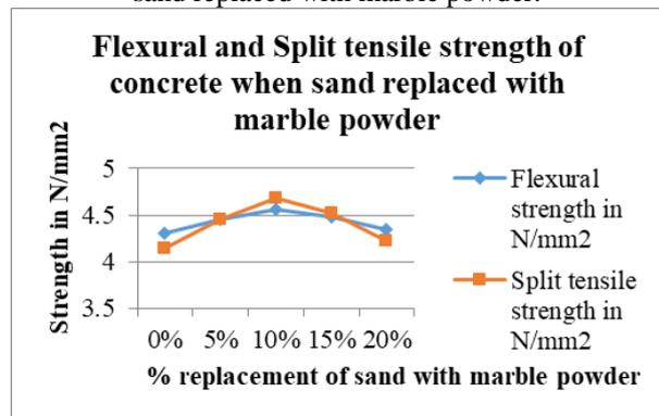
Fig. 9: Indicates the Flexural and Split tensile strength of concrete when sand replaced with marble powder
