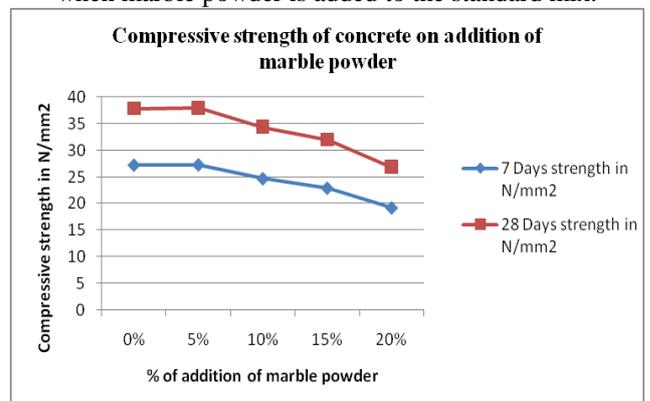
Fig. 5: Indicates the compressive strength of concrete on addition of MP to the standard mix.
