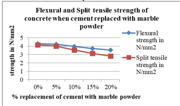
Fig. 5: Indicates the Flexural and Split tensile strength of concrete when cement replaced with marble powder
