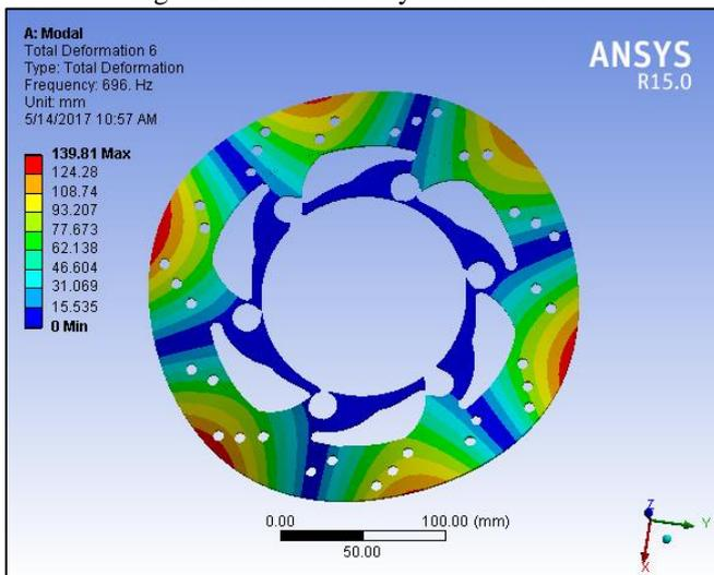
Fig. 8.C: C-Composite at 6<sup>th</sup> node
