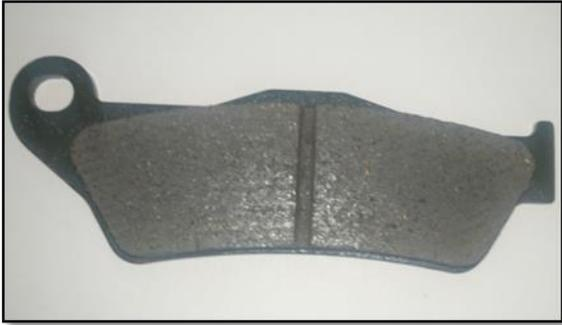
Fig. 5: A Actual brake pads for Bajaj pulsar 180cc
