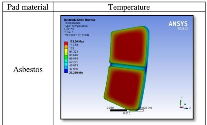
Fig. 6.2: Temperature distribution on brake pads
