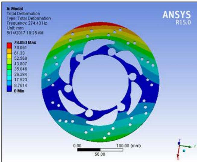
Fig. 8.A: Original Disc at 1<sup>st</sup> node
