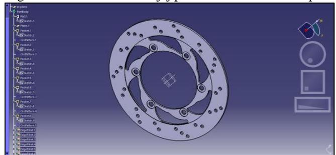
Fig 6: B Modeling of Original disc brake ofPulsar in CATIA
