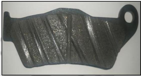
Fig 5: B Modified hatched brake pad for Bajaj 180cc
