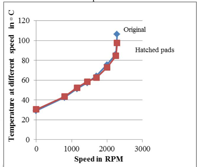
Graph 2: Experimental results for the original brake pads and hatched brake pads
