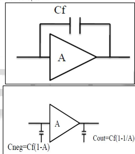
Fig. 1. (a) Negative capacitance implementation using non-inverting amplifier with feedback capacitance. (b) The Miller equivalent circuit of (a). [10]
