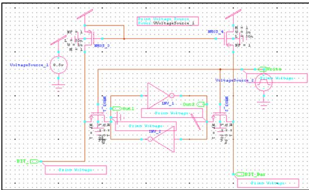
Fig. 3: 6T SRAM read operation
