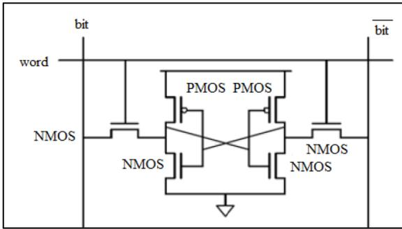
Fig. 2: Architecture of 6T SRAM
