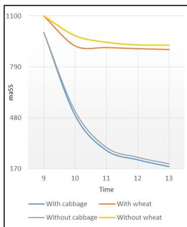
Fig. 2: Variation of loss of moisture for different produce (with and without booster mirror) with time
