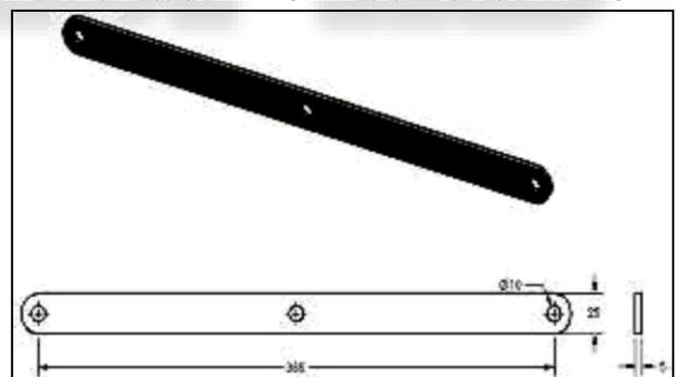
Fig. 5: Dimensions of Link (All dimensions in mm)
