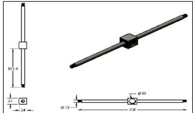
Fig. 4: Dimensions of Nut
