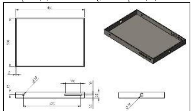
Fig. 1: Dimensions of the Base Plate.
