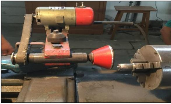
Fig. 3.4: lathe grinder
