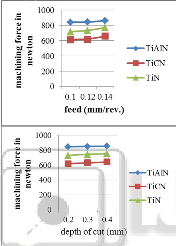
Fig. 5.1: comparison of force with speed, feed and doc Machining force was calculated by:-
