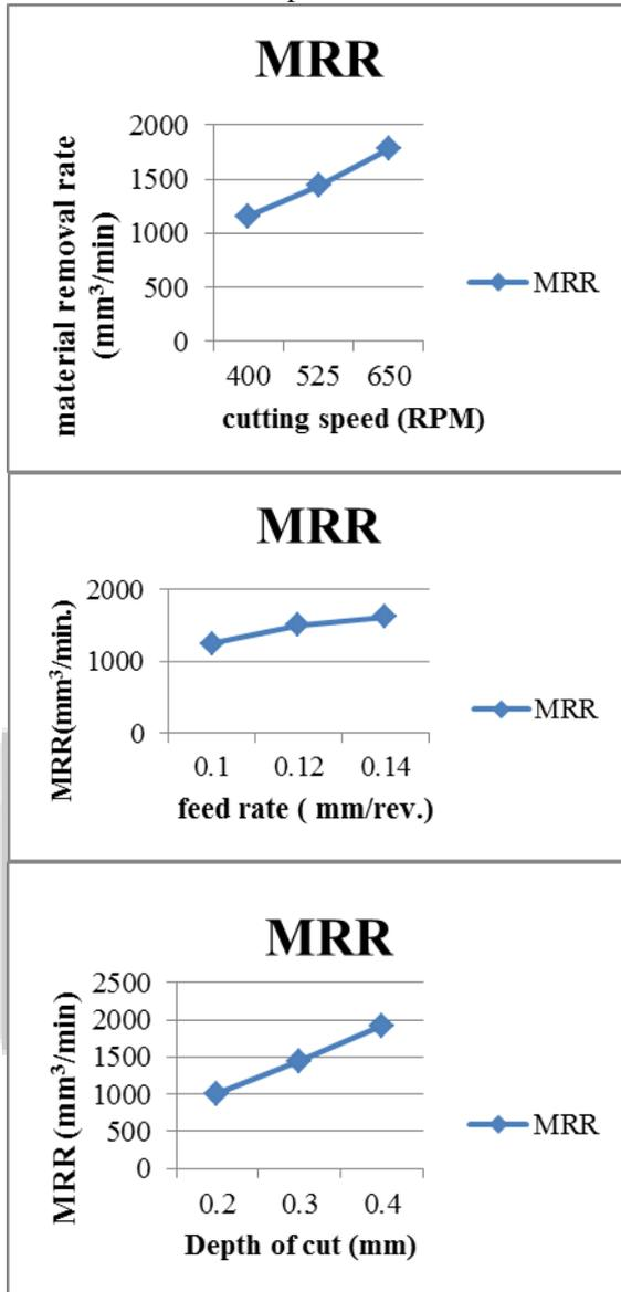
From the above figure it has been observed that the as there is an increase in cutting speed, feed rate and depth of cut material removal rate increased.
