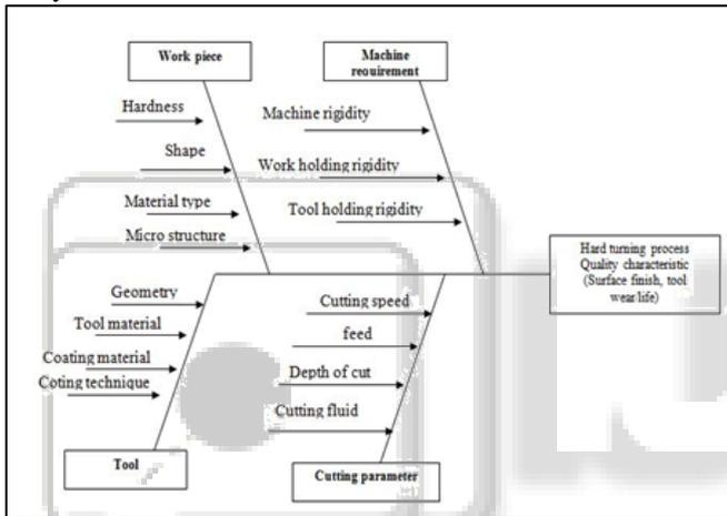
Fig. 2.1: fishbone diagram for hard turning
