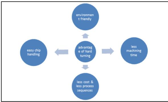
Fig. 3: Advantage of hard turning
