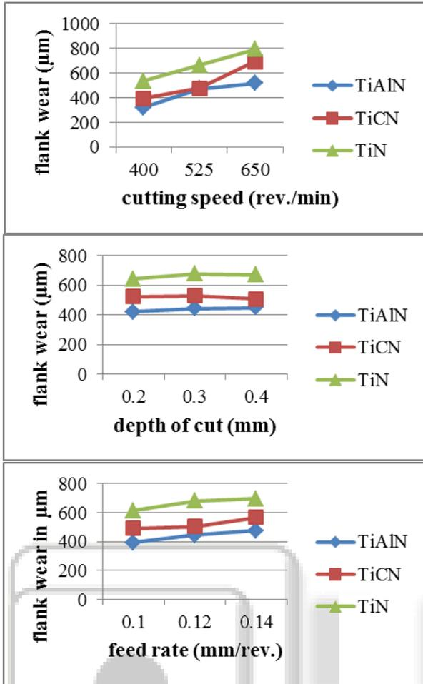
Fig. 5.3: comparison of flank wear of different coating
