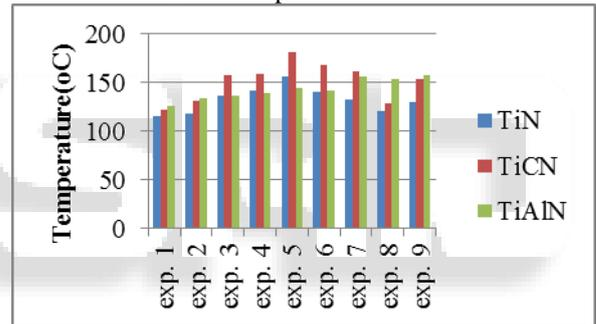
The comparison of Temperature for each coating and each experiment was shown in the graph above. In the graph, sometimes TiCN shows high temperature (experiment 3, 4, 5, 6, and 7) and for the rest experiment TiAlN coating shows high temperature. This temperature depends upon the thermal conductivity of the coating material.
