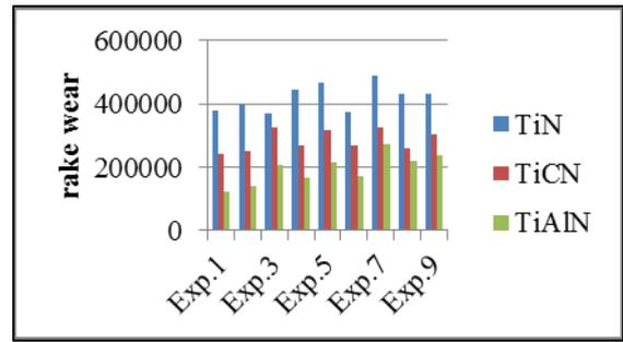
In the above graph rake wear was shown for the each coating and individual experiments. It was observed that the rake wear was highest for the TiN coating followed by TiCN and TiAlN coating.
