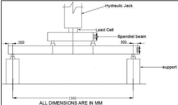
Fig. 8: Test set up
