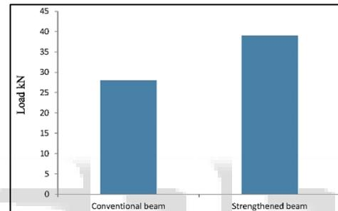
Fig. 11: Comparison of First Crack load
