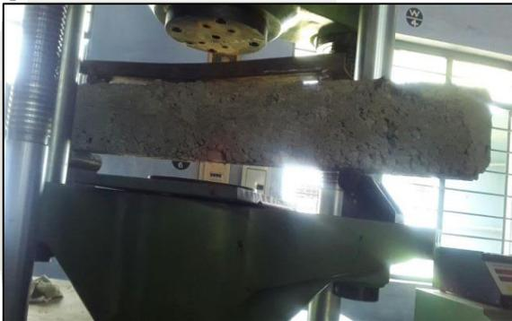
Fig. 9: Testing of conventional beam
