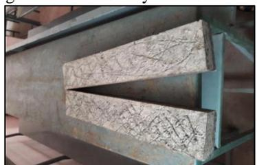
Fig. 5: Finished Sifcon Laminate
