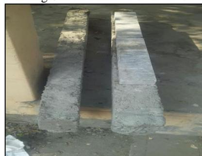
Fig. 7: Conventional and Strengthened beams
