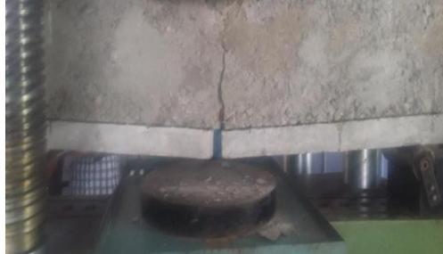
Fig. 14: Failure pattern in strengthened RC beam
