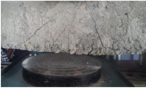
Fig. 13: Failure pattern in conventional beam
