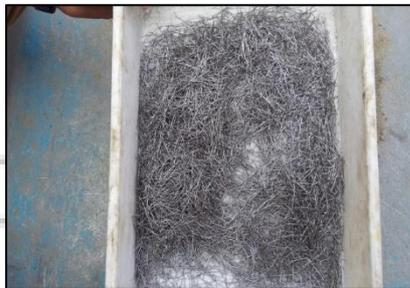
Fig. 1: Hook End Steel Fibre
