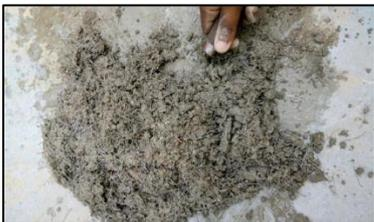
Fig. 4: Cement Slurry with Steel fibre
