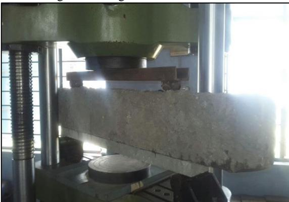
Fig. 10: Testing of strengthened beam
