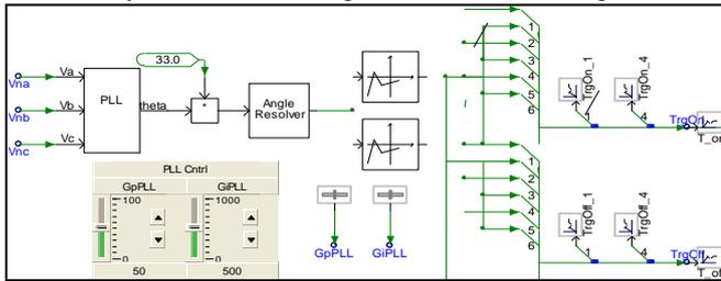
Fig. 3: Generation of carrier signal
