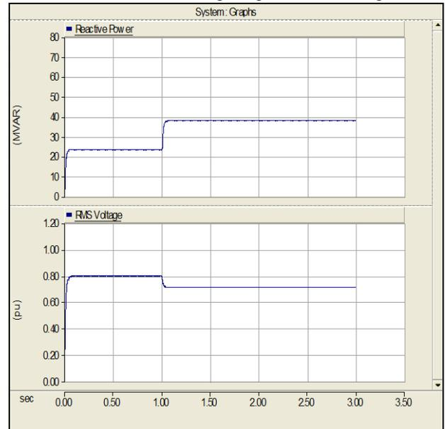
Fig. 6: Simulated waveform without STATCOM
