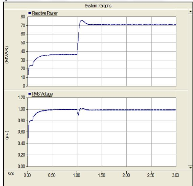
Fig. 7: Simulated waveform with STATCOM
