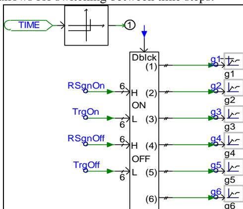
Fig. 5: Generation of firing pulses for STATCOM
