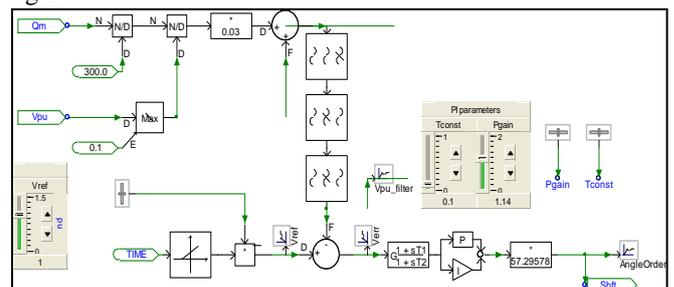
Fig. 2: Voltage control loop
