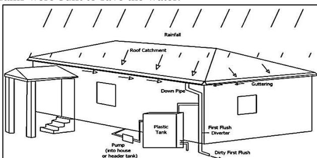
Fig. 1: Example of rain water harvesting system
