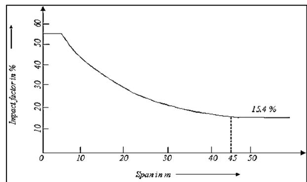
Fig. 2: Impact percentage curve for highway bridges for IRC class A and IRC Class B Loadings
