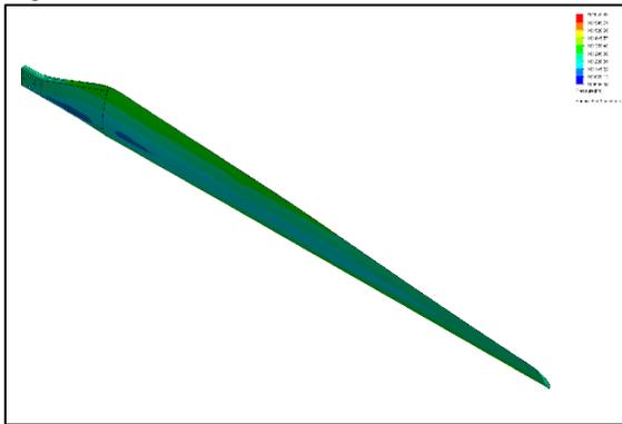
Fig. 4: Surface Pressure Distribution
