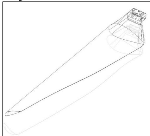
Fig. 2: Wireframe model of Windmill Blade
