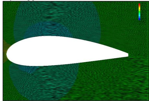
Fig. 7: Pressure cut plot
