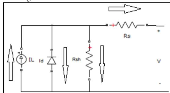
Fig. 1.1: Equivalent Circuit of Solar Cell
