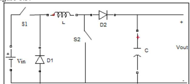
Fig 1.5 Circuit Diagrams Of Buck Boost Converter
