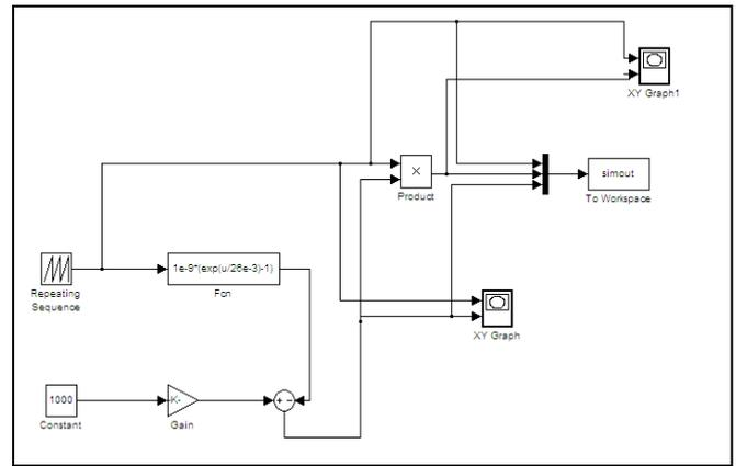
Fig.1.4 Simulink Model of Photovoltaic System
