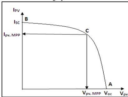
Fig. 1.2: I-V and P-V Characteristics of Photovoltaic System
