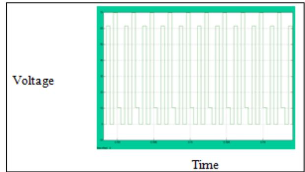
Fig. 1.12: Simulation waveform of buck boost converter at 60V when the input voltage is 74V.
