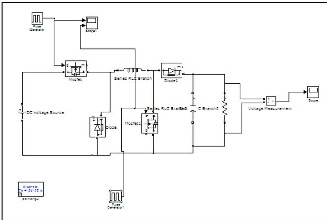
Fig.1.6 Simulink Model of Buck Boost Converter
