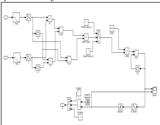
Fig.1.7.Simulink Model Of Maximum Power Point Tracking
