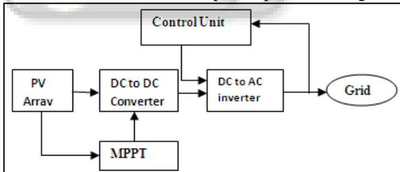
Fig. 1.3: Grid Connected Photovoltaic System
