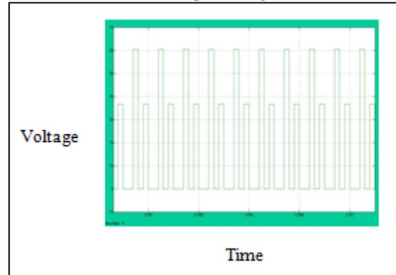
Fig. 1.13: Simulation waveform of buck boost converter at 60V when the input voltage is 45V.
