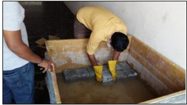
Fig. 3: Immersion of specimens in acid tank
