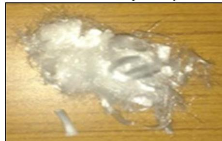
Fig. 1: Polypropylene Fibers
