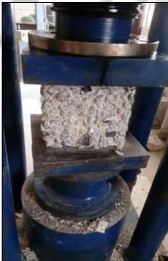
Fig. 2: Testing of cubes for Compressive strength
