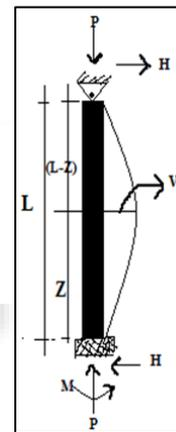
Fig. 2: Free body diagram of one side fixed and other side pinned column
