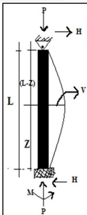
Fig. 3: Free body diagram of one side fixed and other side pinned column
