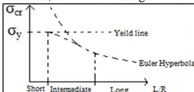
Fig. 1: Classification of Column based on Slenderness ratio.
