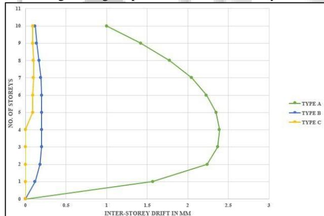
Fig. 10: Inter-storey drift vs No. of storeys
