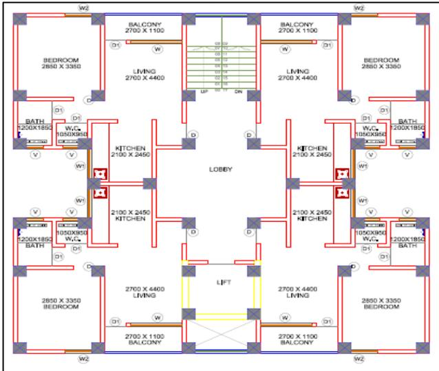
Fig. 1: Type A Typical layout
