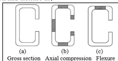
Fig. 1: Buckling of C-section elements.
