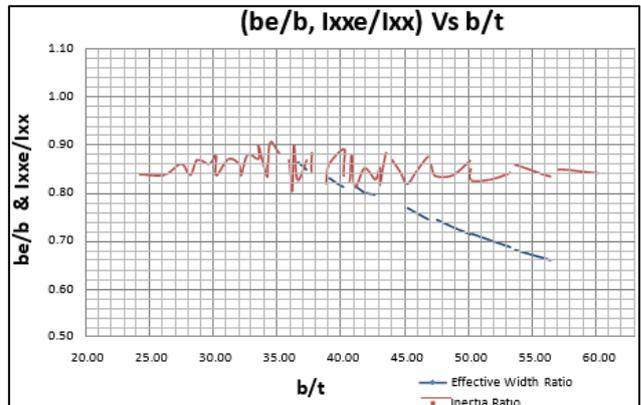
Fig. 5:  $b_e/b$  versus  $b/t$  and  $I_{xxe}/I_{xx}$  versus  $b/t$  for Indian code.
