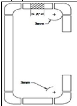
Fig. 3: Element for calculation of sectional properties
