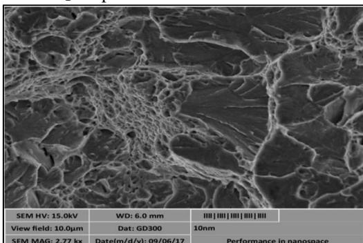
Fig. 3: Scanning and Transmission electron micrographs of the designed steel (grade C300) after oil cooling at temperature 480°C.
