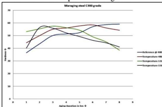
Fig. 1: Effect of aging time and temperature on the hardness of a maraging steel grade C300
