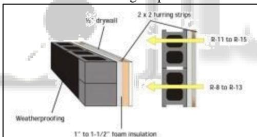
Figure 2: Interior Foam Wall Insulation
