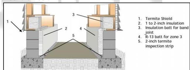
Fig. 5: Insulated, Sealed Crawl Space Walls
