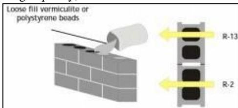
Fig. 1: Insulating Concrete Block Cores
