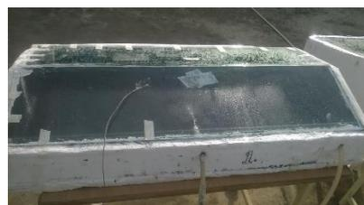
Fig. 1: Experimental setup of non-conventional double slope solar still.
