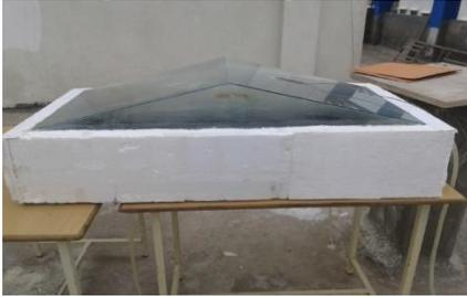
Fig. 2: Non-conventional still with granite pieces and saline water
