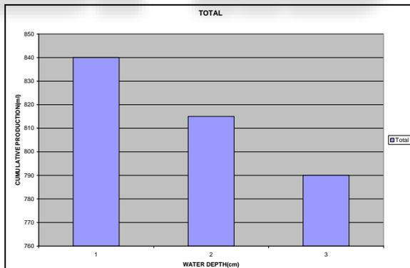
Fig. 5: Cumulative production with respect to depth of water for aluminum
