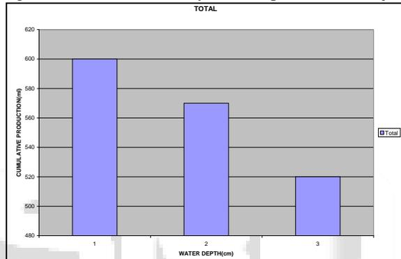
Fig. 4: Cumulative production with respect to depth of water for modified still
