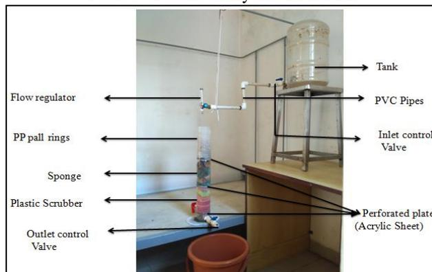
Fig. 3: Hybrid Aerobic Trickling Filter Bed Reactor
