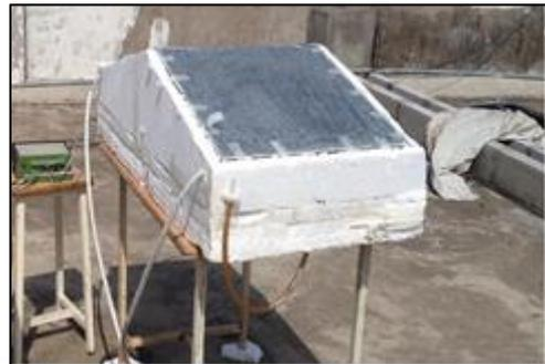
Fig. 3: width wise double slope solar still Non-conventional solar still (modified)
