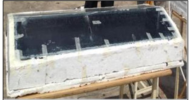
Fig. 2: length wise double slop solar still Conventional solar still
