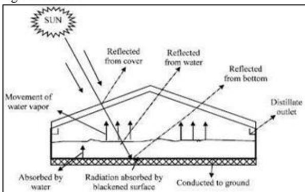
Fig. 1: Double slope solar still[9]
