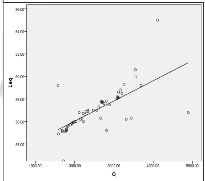
Fig. 4: Total traffic volume (Q) in regard to equivalent noise level ( $Leq$ )
