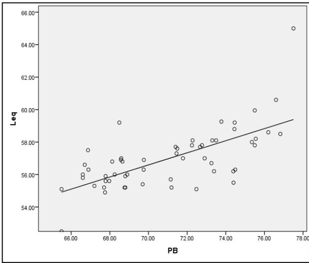
Fig. 5: Percentage of two wheelers (PB) in regard to equivalent sound pressure level (Leq)
