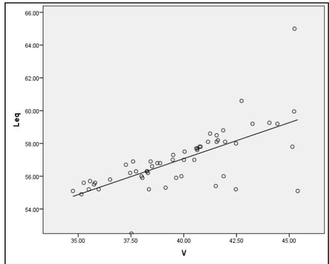
Fig. 3: Spot Speed of Vehicles (V) in regard to equivalent noise level ( $Leq$ )
