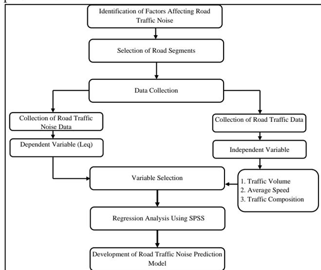
Fig. 1: Methodology for Development of Road Traffic Noise Prediction Model
