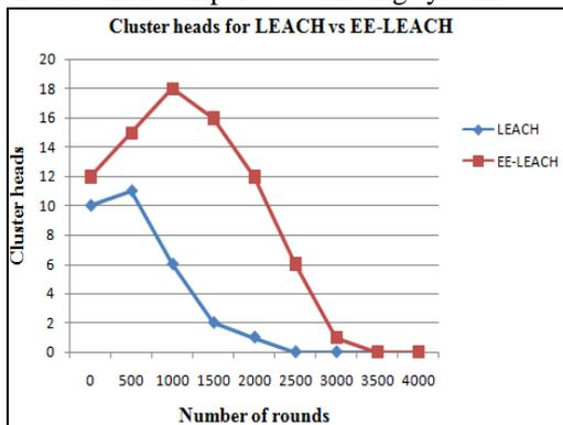
Fig. 3: Cluster heads for LEACH vs EE-LEACH
