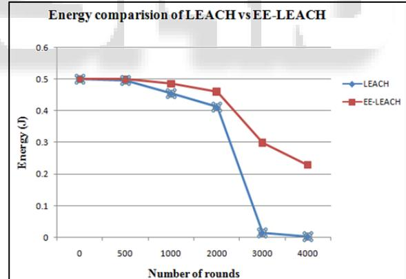
Fig. 5: Energy comparison of LEACH vs EE-LEACH
