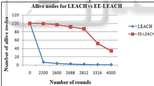
Fig. 2: Alive nodes for LEACH vs EE-LEACH
