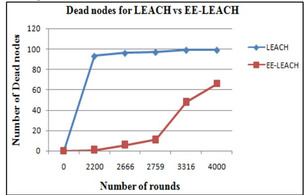
Fig. 4: Dead nodes for LEACH vs EE-LEACH
