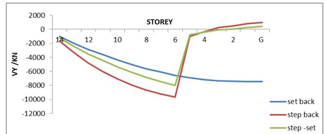
Fig. 12: Variation of Storey Shear for Three Buildings under Load combination (0.9 DL + 1.5 ELY)
