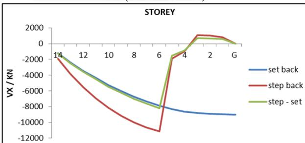
Fig. 10: Variation of Storey Shear under Load of combination (0.9 DL + 1.5 ELX)
