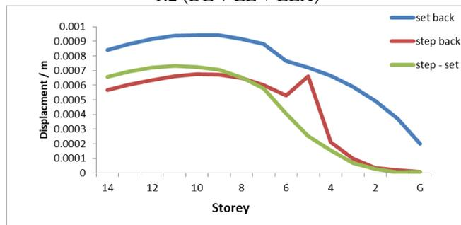
Fig. 6: Variation of Storey Drift for Load of combination (0.9DL+1.5 ELX)
