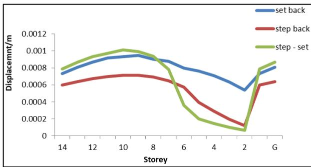
Fig. 7: Variation of Storey Drift in Y Direction under Load of combination 1.2 (DL+LL+ELY)
