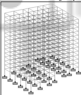
Fig. 3: Isometric view Step-set Back Building
