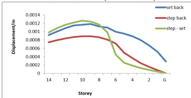
Fig. 8: Variation of Story Drift Storey in Y direction under Combination Load (0.9DL + 1.5 ELY)
