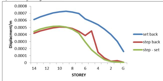
Fig. 5: Variation of Storey Drift under Load of combination 1.2 (DL + LL + ELX)
