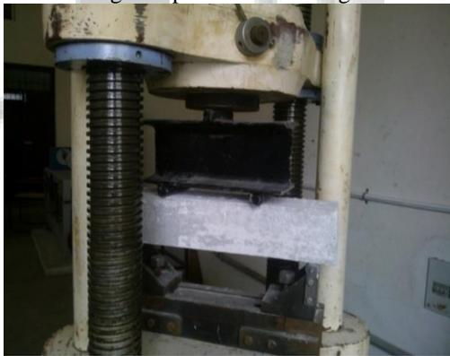
Fig. 4: Flexure Set Up
