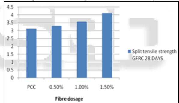
Fig. 6: Split tensile strength of GFRC at 28 days curing
