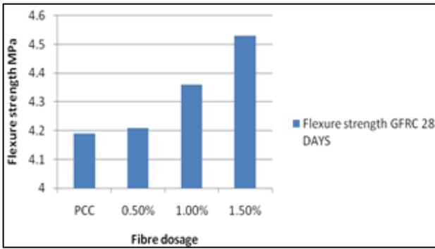
Fig. 7: Flexure strength of GFRc at 28 days curing
