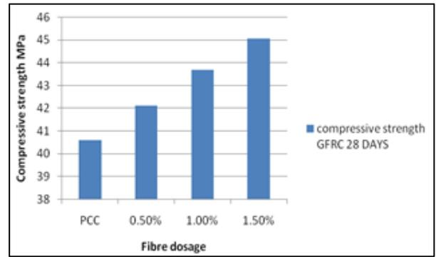
Fig. 5: Compressive strength of GFRC at 28 days curing
