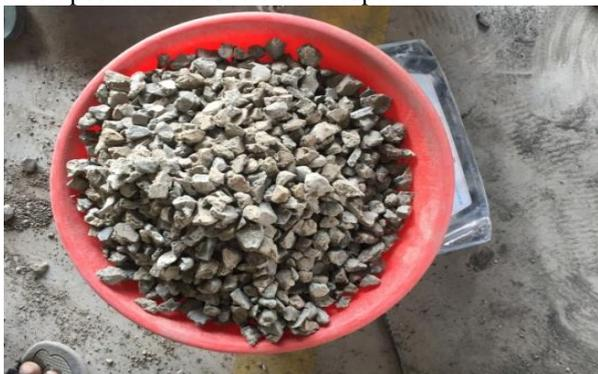
Fig. 3: Recycled Aggregate
