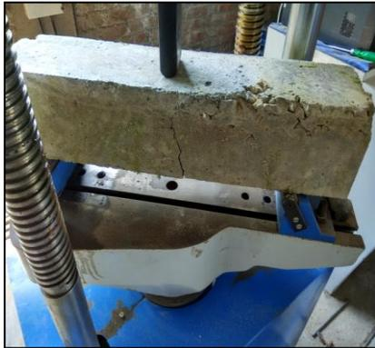
Fig. 6: Setup of flexural strength on UTM
