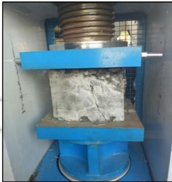
Fig. 4: Setup of Compressive Strength Testing Machine
