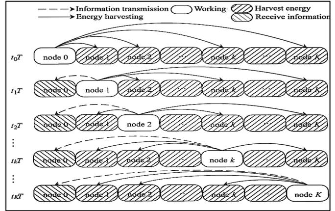
Fig. 3: The timing diagram of CEH.
