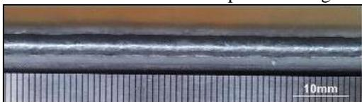
Fig. 4: Appearance of weld under optimized condition
