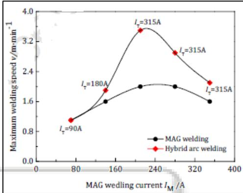
Fig. 2: Comparison between conventional and hybrid welding speed at different MIG currents.
