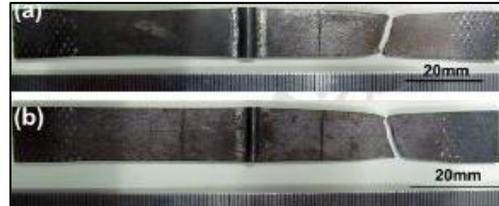
Fig. 5: Fractures of tensile specimens: (a) MIG welding specimen, (b) TIG-MAG hybrid arc welding specimen
