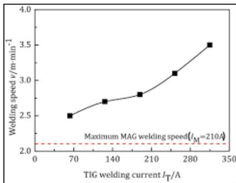
Fig. 6: Hybrid arc welding speed at different TIG welding currents
