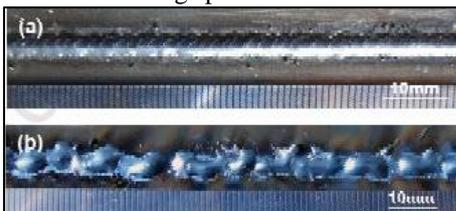
Fig. 3: Weld appearance at 70A MIG welding current (a) conventional MIG weld, (b) TIG-MIG
