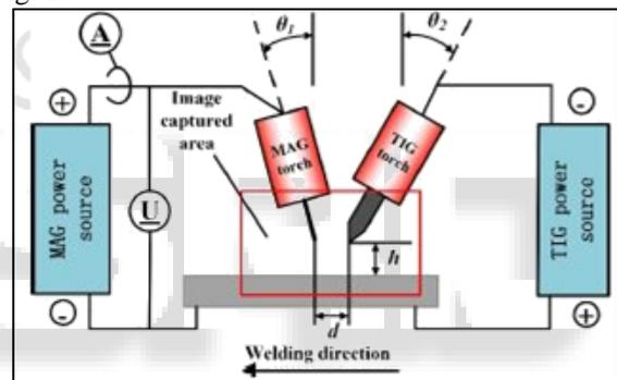
Fig. 1: Experimental setup for TIG-MIG hybrid welding
