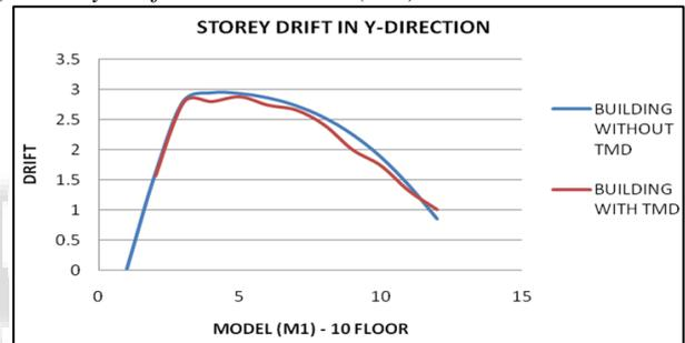
Fig. 9: Storey Drift in Y-Direction (M1)
