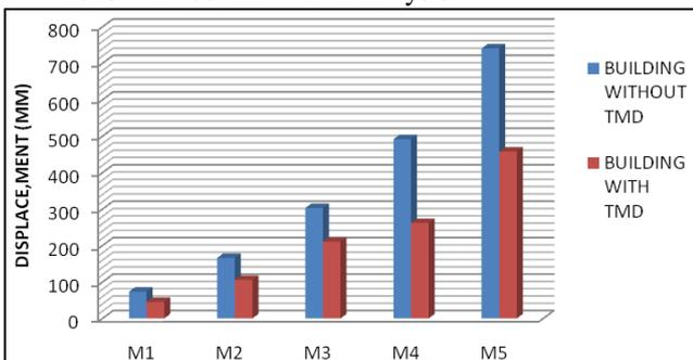
Fig. 7: Maximum displacement in Y-Direction
