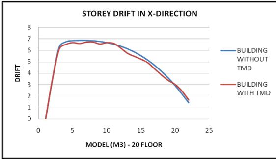
Fig. 12: Storey Drift in X-Direction (M3)
