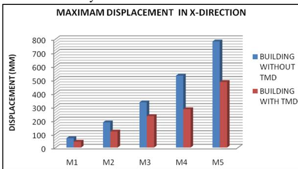
Fig. 6: Maximum displacement in X-Direction
