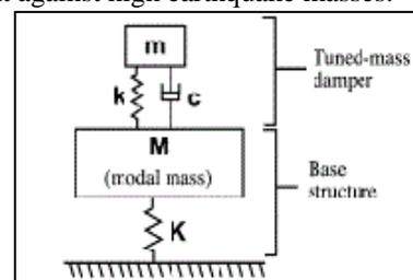
Fig. 1: A schematic representation Tuned Mass Damper (TMD)
