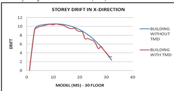
Fig. 16: Storey Drift in X-Direction (M5)
