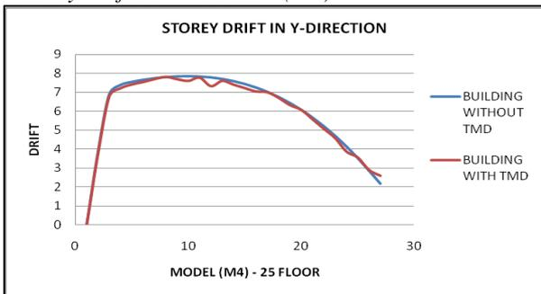
Fig. 15: Storey Drift in Y-Direction (M4)
