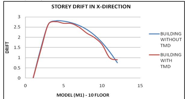
Fig. 8: Storey Drift in X-Direction (M1)
