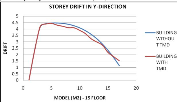
Fig. 11: Storey Drift in Y-Direction (M2)
