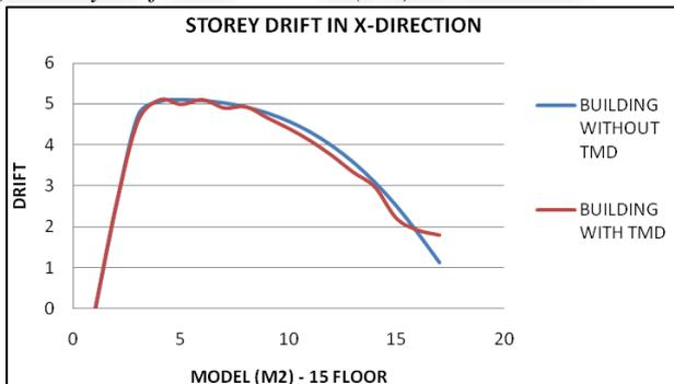
Fig. 10: Storey Drift in X-Direction (M2)
