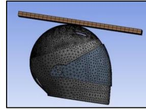
Fig. 4: Meshed helmet structure
