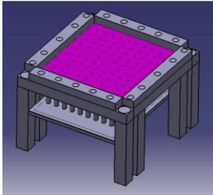
(a) Proposed Setup with clamped Sheet
