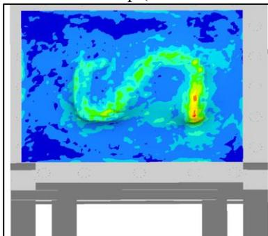
(b) Flexible Hydraulic Support (Max Stress 248 MPa)
