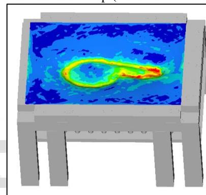
(b) Flexible hydraulic support setup (Max Stress 218 MPa)
