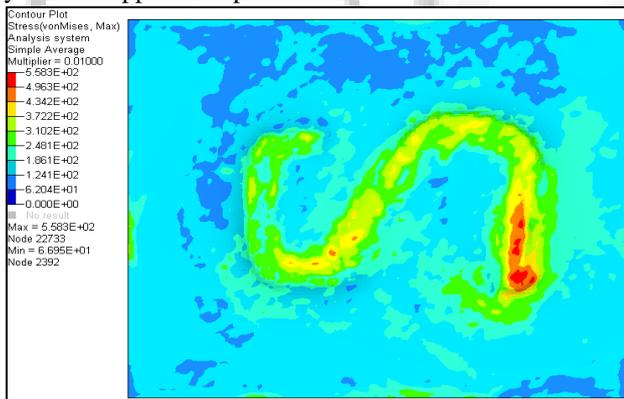
(a) Conventional Setup (Max Stress 496 MPa)
