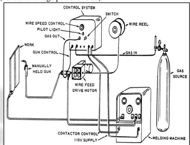
Fig. 1.1: Metal Inert Gas Welding (MIG)
