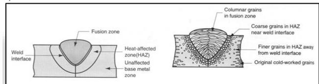
Fig. 1.2: Zones in Welded Joint
