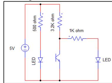
Fig. 7: Photo detector Circuit
