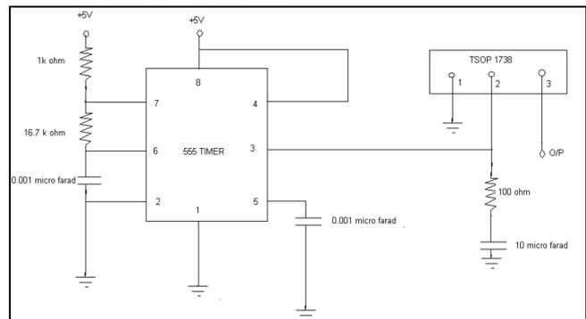
Fig. 6: IR Transmitter and Receiver circuit
