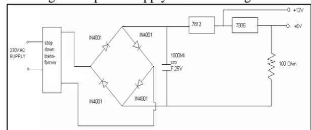
Fig. 2: Circuit diagram of Power supply
