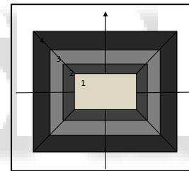
Fig. 1: Decomposition of image into subbands
