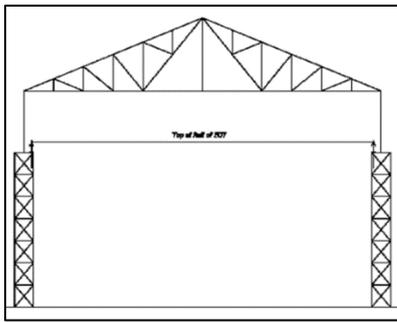
Fig. 2: Conventional steel building frame
