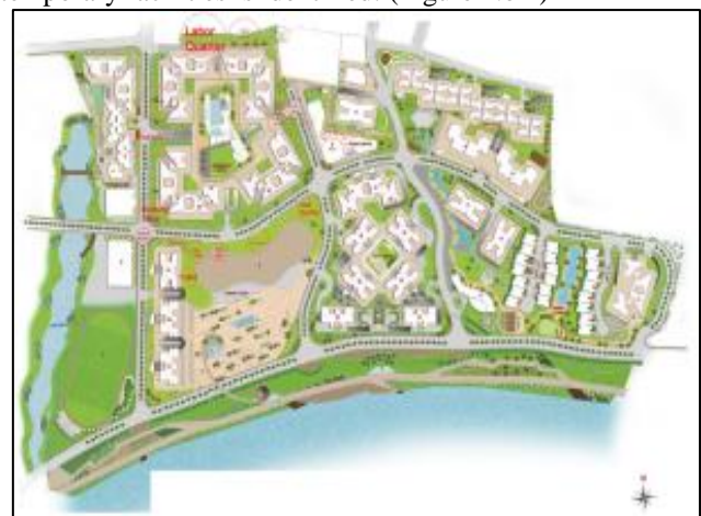
Fig. 4: Initial Location Of Temporary Facilities.
