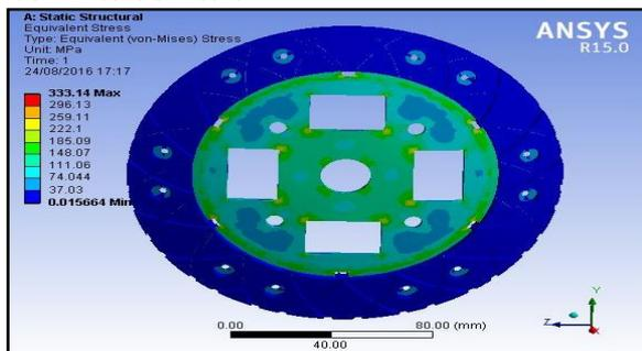
Fig. 8: Von-misses stresses for sunburst grooves
