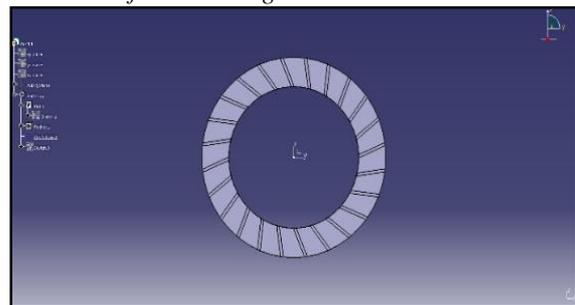
Fig. 3: 3D Friction plate with 23° Inclined groove
