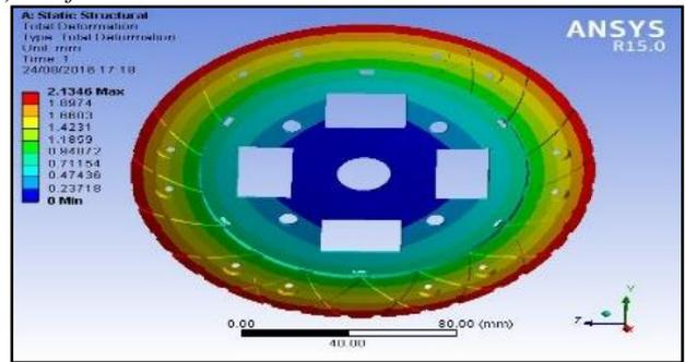
Fig. 9: Deformation for sunburst grooves
