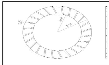
Fig. 1: 2D Friction plate with 23° Inclined grooves
