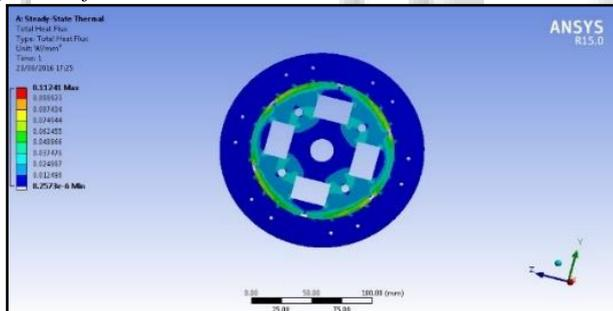
Fig. 7: Heat Flux for 23° inclined grooves
