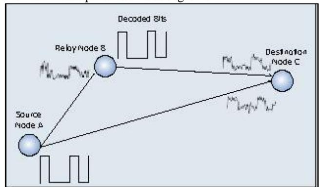
Fig. 1: Decode and Forward technique
