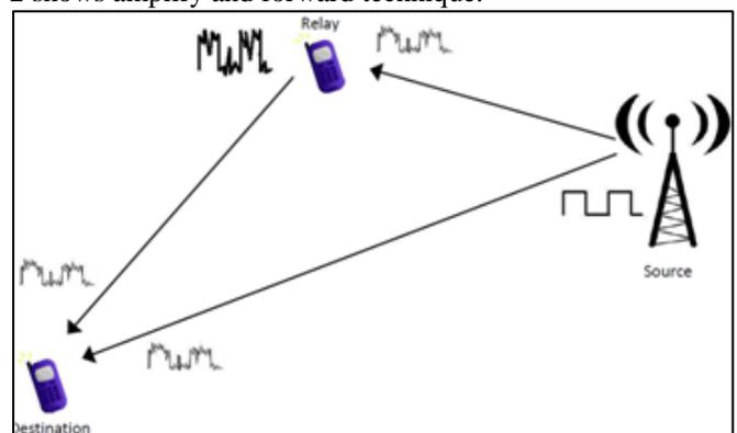
Fig. 2: Amplify and forward technique
