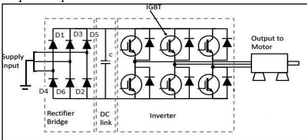
Fig. 2: Basic diagram of variable frequency drive
