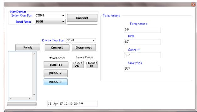
Fig. 8: Parameters at speed 3 on application software.
