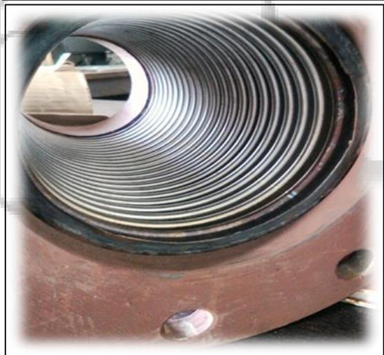
Fig. 19: Metallic Flexible Hose Joint
