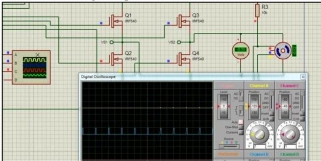
Fig. 2: Motor Voltage Variation at 25% PWM Speed
