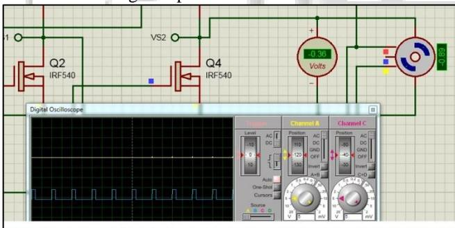
Fig. 4: Motor Voltage Variation at 50% PWM Speed
