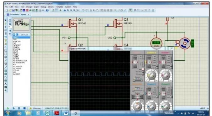
Fig. 6: Motor Voltage Variation at 75% PWM Speed
