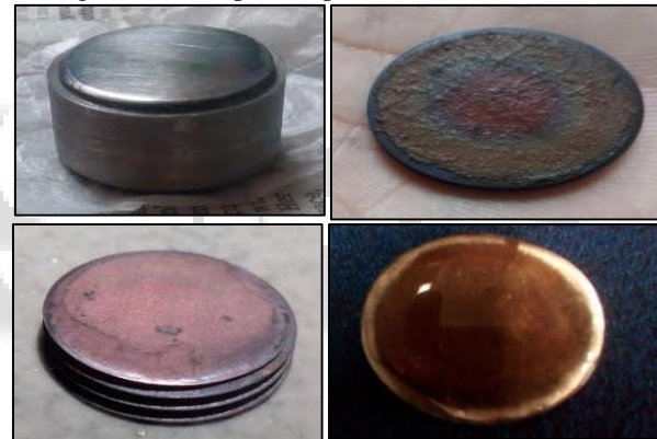
Fig. 5: Metallic fixture and clad surface
