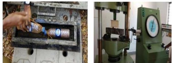
Fig. 4: Study of flexure strength characteristic behaviour
