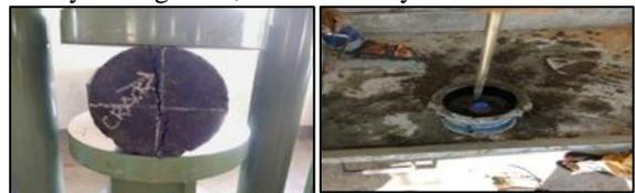
Fig. 3: Study of split tensile characteristic behaviour
