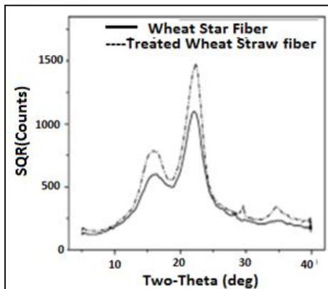
Fig. 2: XRD patterns of the untreated and treated wheat straw fiber.
