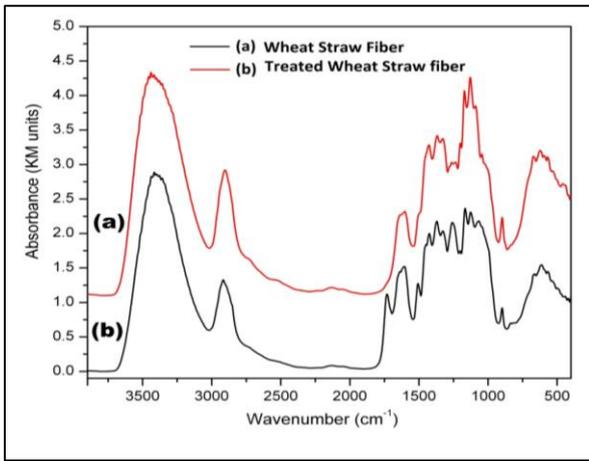
Fig. 1: FT-IR spectra of (a) an untreated wheat straw and (b) chemically treated wheat straw.
