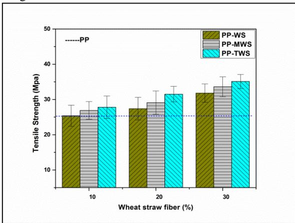
Fig. 5: Tensile Strength of PP/Wheat straw fiber composites
