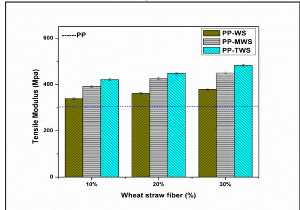
Fig. 7: Tensile Modulus of PP/Wheat straw fiber composites
