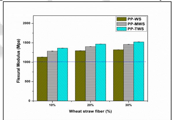
Fig. 8: Flexural Modulus of PP/Wheat straw fiber composites
