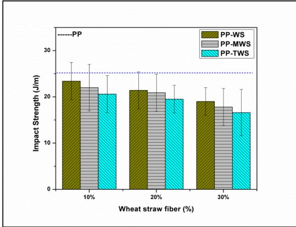
Fig. 9: Impact Strength of PP/Wheat straw fiber composites
