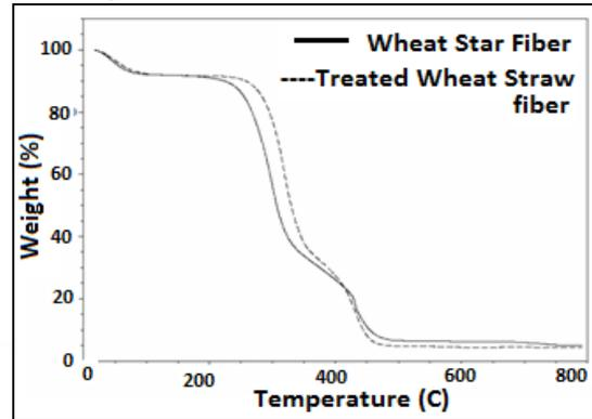
Fig. 3: TGA of the untreated and treated wheat straw fiber
