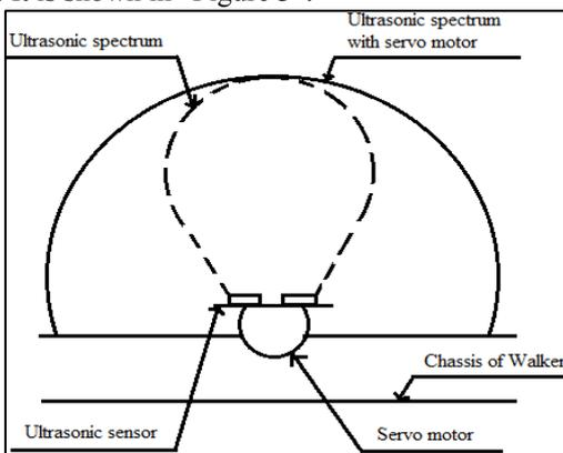
Fig. 3: Ultrasonic sensor obstacle detection scheme
