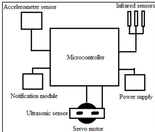
Fig. 2: Block diagram for smart walker
